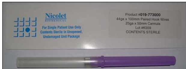
Fig. 7 Fine wire electrode. 44ga × 100 mm Paired Hook Wires in a 25ga × 50 mm Cannula.
