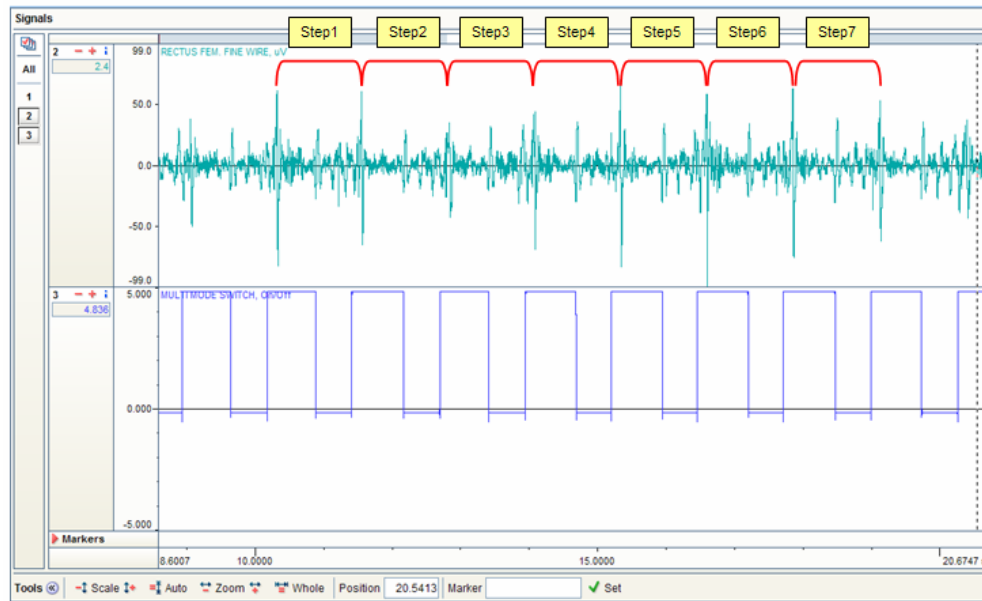
Fig. 14 Fine wire recording of Rectus Fem. (upper channel) in a treadmill walking trial. The cable motion artifact has repetitive nature directly related to the gait event (see foot switch signal – lower channel).
